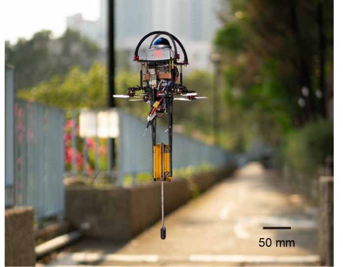
Fig. 1. A 220 g thrust-based hopping robot constructed from a quadcopter (160 g) and a passive leg (60 g) demonstrating an ability to carry a 730 g LiDAR payload for mapping applications. Despite a thrust limit of only 440 g, the hopper is able to carry as much as 2 kg.
